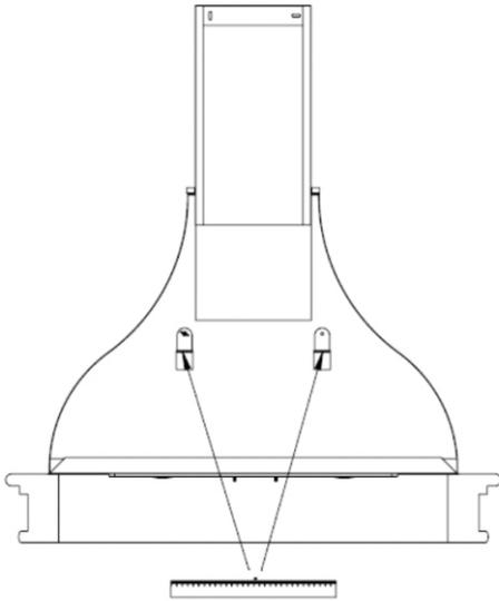
2. Place the chimney (5) fixing the plastic bar (6) to the wall
