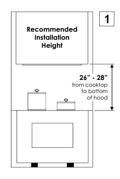
Insert hood into cabinet, and secure with screws.
