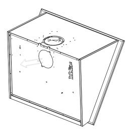
The Quest range hood is equipped with a reversible blower mount that allows the user a choice of vertical or horizontal ducting (rear exhaust). A removable knock-out plate is provided on rear of unit.
