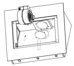
Step 2: remove blower, then remove the knock-out plate on rear wall of range hood. Rotate the blower 90 degrees and insert into the hole left by the knock-out plate.
