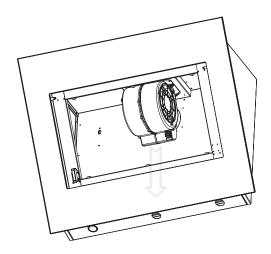
Step 1: disconnect 1 plug (on bottom of blower), then remove 4 screws holding the blower.
