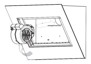
Step 3: secure the blower with the 4 screws removed in Step 2, and reconnect the plug. Connect the range hood to 110V AC power supply and test its operation **prior** to continuing installation.
