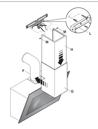
**OPTIONAL - Step 4:** If using a chimney cover, attach the cover mounting bracket to wall, then attach the cover section(s).
