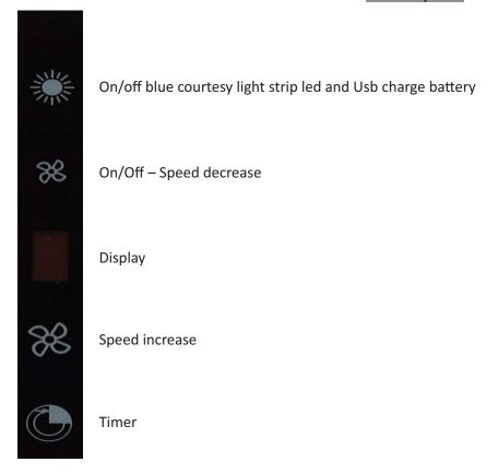
Sun: ON/OFF courtesy blue light on the bar led and Usb charge battery. To switch on touch the blue light.
