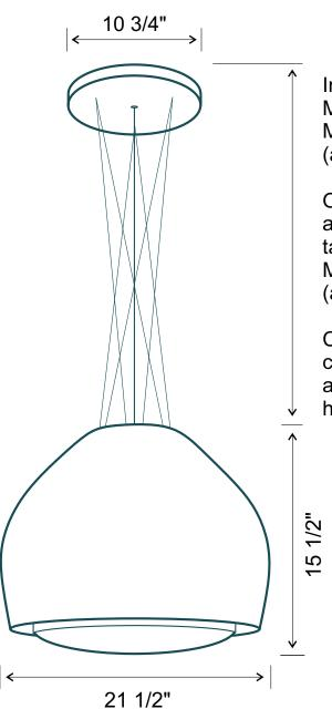
Includes 6 x 43" long strings. Min usable length 15 3/4" Max usable length 40 1/2" (after mounting)
