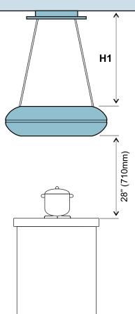
Includes 6x43" long wires. Min usable length 15 3/4" Max usable length 40 1/2" (after mounting)
