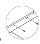
Insert hood body into cabinet, and secure with 4 screws (2 on each side).
