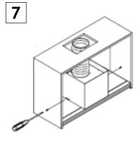
Insert, but do not tighten completely, 1 screw into each side of the top cover.
