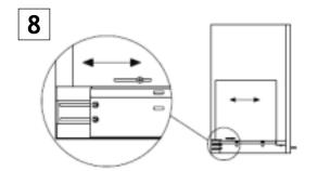
Adjust position of top cover as needed, using the adjustment screw & slot. Secure the adjustment screw when finished.
