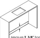
Measure **2** 3/8" from bottom of cabinet, for filler panel position
