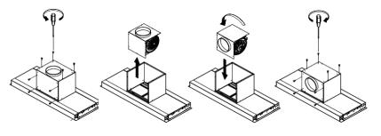
**NOTE:** The bottom of the hood should be even with, or slightly below, the bottom of the cabinet - NOT above it. Front of hood should line up with door.
