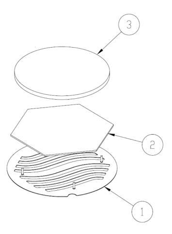
In case of filtering hood remove 4 screws in the aluminium filter (2) place and push down on it the carbon filter (3) and then join all together.
