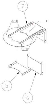
2. Drill the wall in order to fix the support (7) by the provided 4 expansion wall plug
