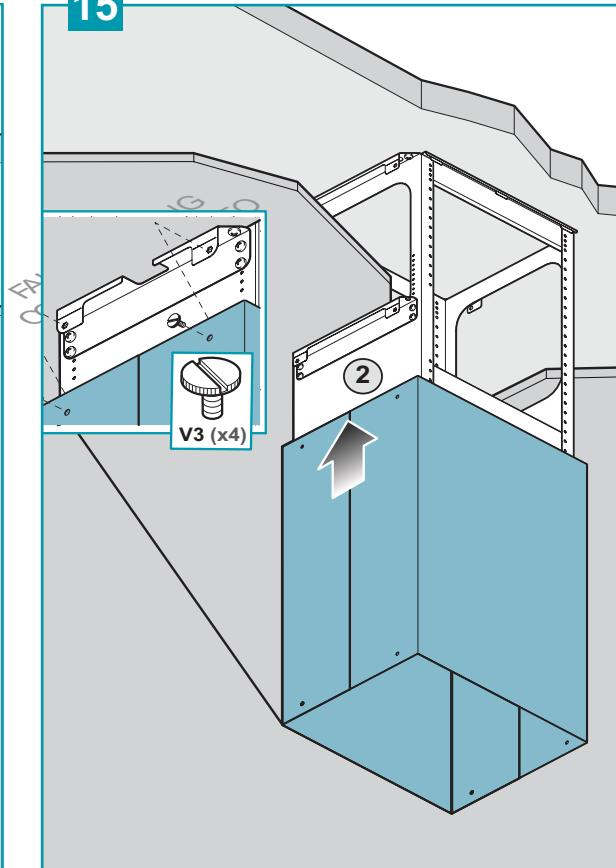
**Motor chamber installation (16);
